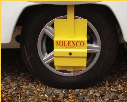
Slide the Milenco front cover with top strap over the wheel in a horizontal position, avoiding the wheel arch of the vehicle.
