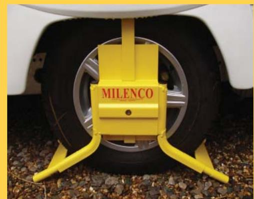
Lock wheelclamp by rotating the key 90 degrees anti-clockwise, and then remove your key.
