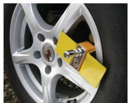
Turn key to lock. The parked position of the holes in the wheel will determine how taught you will be able to lock the wheelclamp on. This however does not effect the level of security.
