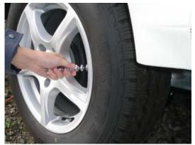
Tug hard on the chrome end visable through the front of the wheel to ensure its as tight as possible.
