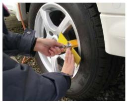
Insert key and release the lock. Fit the lock into the clamp plate and insert into the chrome section at the front of the wheel.
