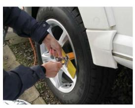
Push the lock and plate to the back of the chrome section and let it slot into the tightest notch possible.
