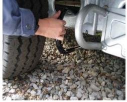
Whilst holding the short black section of the wheelclamp (with the long chrome section at the bottom, pointing towards the wheel) insert the short black section into the chassis hole. Rotate the clamp back on itself so the long chrome section is now on top. Holding the end of the chrome section push back into the chassis and then move behind wheel and feed the chrome section back out through the hole in the wheel.
